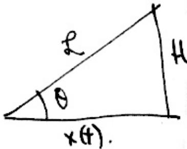
$$\text{Then, computing the derivative w.r.t. time: } \frac{d}{dt}(\tan \theta(t)) = \frac{d}{dt}\left(\frac{H}{x(t)}\right)$$
